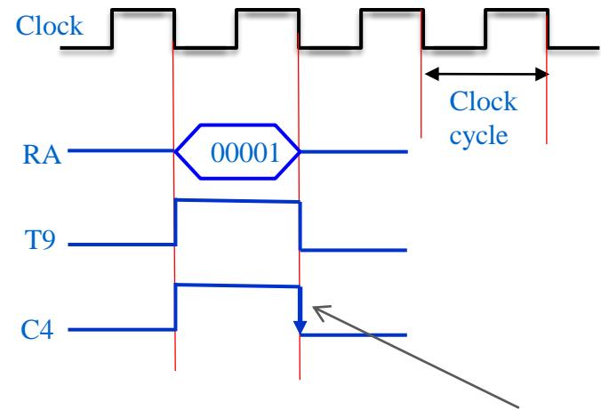
The data is loaded on RT1 on the falling edge.
